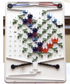
Figure 3.26: The game “Turing Tumble” contains an implementation of logical gates using marbles.
