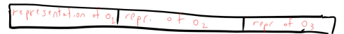
Figure 2.9: If we have a prefix-free representation of each object then we can concatenate the representations of k objects to obtain a representation for the tuple (o_0, \dots, o_{k-1}) .
