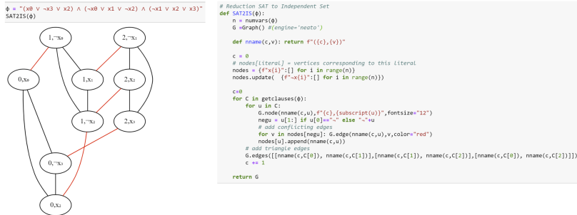
Figure 13.5: The reduction of 3SAT to Independent Set. On the righthand side is Python code that implements this reduction. On the lefthand side is a sample output of the reduction. We use black for the “triangle edges” and red for the “conflict edges”. Note that the satisfying assignment x^* = 0110 corresponds to the independent set (0, \neg x_3), (1, \neg x_0), (2, x_2) .
