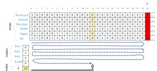
**Figure 12.11:** We simulate a  $T(n)$ -time NAND-TM program  $P'$  with an *oblivious* NAND-TM program  $P$  by adding special arrays  $Atstart$  and  $Atend$  to mark positions 0 and  $T - 1$  respectively. The program  $P$  will simply “sweep” its arrays from right to left and back again. If the original program  $P'$  would have moved  $i$  in a different direction then we wait  $O(T)$  steps until we reach the same point back again, and so  $P$  runs in  $O(T(n)^2)$  time.
