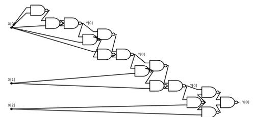
**Figure 12.10:** A NAND circuit for  $XOR_3$  obtained by “unrolling the loop” of the NAND-TM program for computing  $XOR$  three times.
